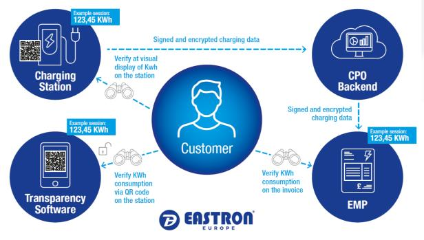
After the charging session, the charger generates signed encrypted data to the CPO (Charge point operator, the CPO will then send the signed and encrypted charging data to the EMP (e-mobility provider) which then creates the invoice for the customer.
