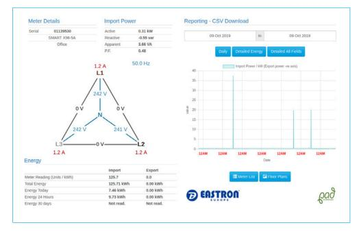
In this view the user is able to interrogate information such as line to line voltages, reactive power, power factor and mains frequency, to allow them to diagnose issues with individual power supplies in the network.
